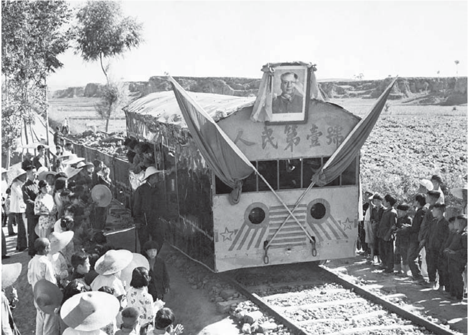
Banners and a portrait of Communist Party Chairman Mao Zedong adorn the front of this strange-looking freight train making its first run in Yuxian County, Shanxi Province. According to information supplied by the Chinese Communists, the 125-mile railroad was built by the people of the county to carry coke to the Yuhsien power equipment plant. The locomotive, powered by a converted automobile engine, pulled six cars, each loaded with three tons of coke, August 5, 1958. (Bettmann/Corbis)
